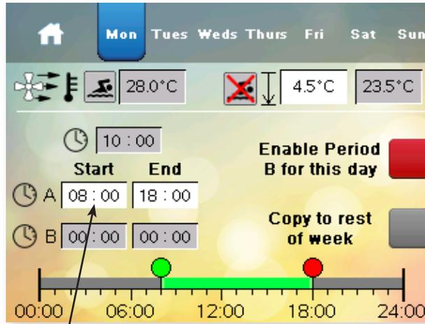
If a second occupied period is required enable this button. Times in the second period can be entered in B.
