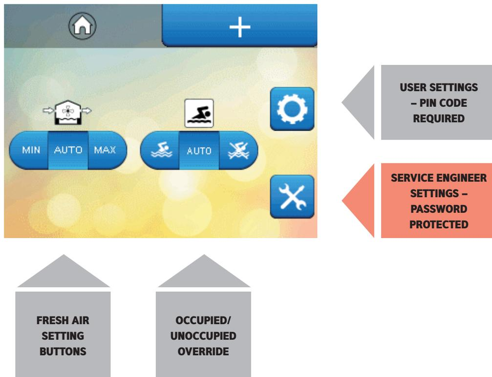
**4. Fresh air setting (where optional fresh air module is fitted)**
