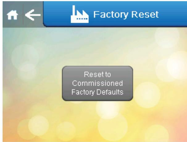
If the settings have been changed in a way that makes the Variheat behave in an unusual way, the original commissioned settings can be restored by pressing the Reset to Commissioned Factory Defaults button on this screen. After this has been pressed a confirmation appears, pressing again completes the reset.
