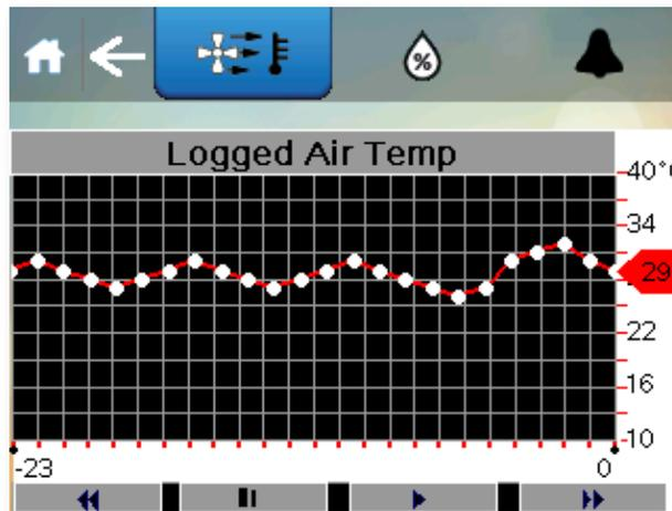
Pressing the buttons brings up a graph of the selected parameter. Choose from Air temperature, Humidity, Water temperature and Alarms. The display is marked up in hours and shows the past 72 hours of activity.
