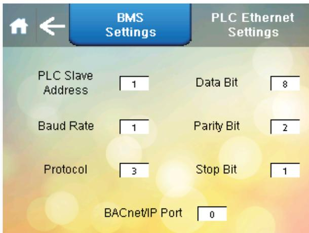
This screen contains settings related to BMS connectivity when using Modbus/RTU and BACnet MS/TP through the spare RS485 port. The factory default settings are shown. If connecting using BACnet/IP, see the PLC Ethernet Settings screen on page 29.
