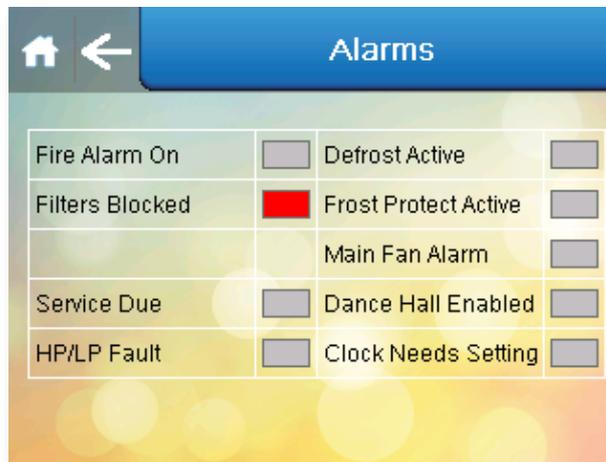
The Alarms screen displays warnings or faults with the Variheat, indicated by a red highlight. The example above indicates that there is a problem with the air filter that should be investigated.
