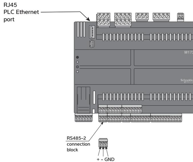
In addition to screen mirroring to the touchscreen (see section 2.1 Advanced Settings), the following options for connecting a BMS are included as standard.
