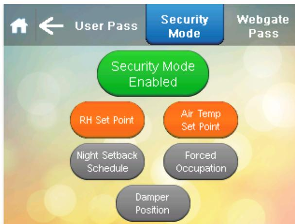
Toggles between Security Mode Enabled and Security Mode Disabled
