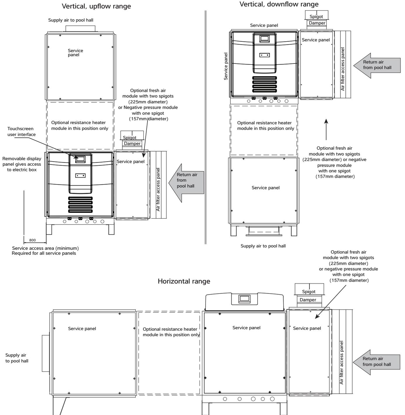
All ambient air ducting should be suitably insulated if plant room temperatures are significantly different from ambient, particularly where the plant room is at pool conditions. Spring return dampers are recommended for exhaust and fresh air ductwork in installations with sub zero ambient temperatures, in case of power failure.
