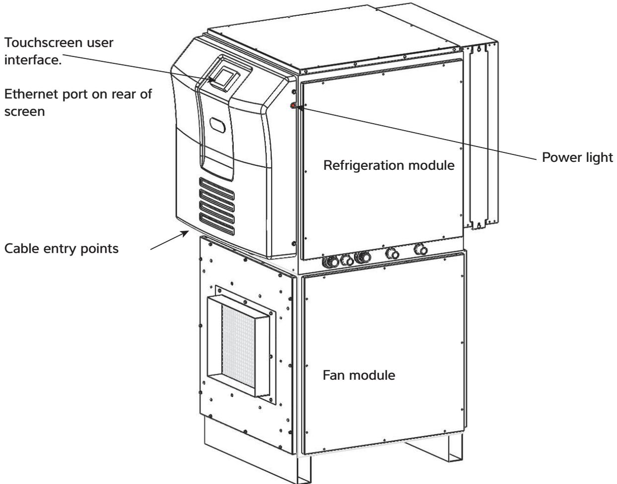
Power light – when illuminated red, power is connected to the Variheat.
