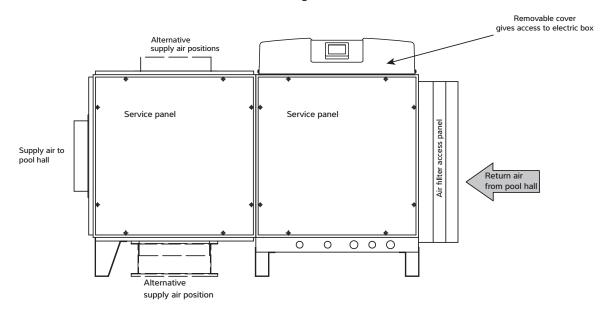
All ambient air ducting should be suitably insulated if plant room temperatures are significantly different from ambient, particularly where the plant room is at pool conditions. Spring return dampers are recommend for exhaust and fresh air ductwork in installations with sub zero ambient temperatures, in case of power failure.
