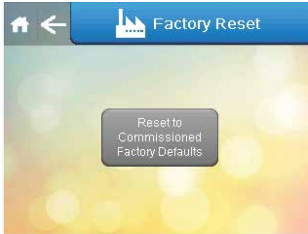
If the settings have been changed in a way that makes the Delta behave in an unusual way, the original commissioned settings can be restored by pressing the Reset to Commissioned Factory Defaults button on this screen. After this has been pressed a confirmation appears, pressing again completes the reset.
