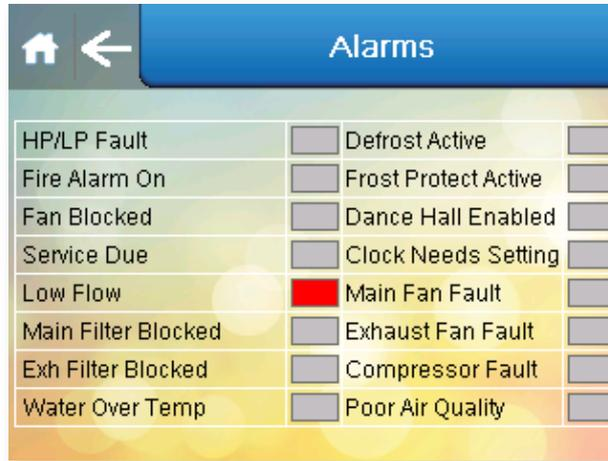
The Alarms screen displays warnings or faults with the Delta, indicated by a red highlight. The example above indicates that there is a problem with the pool water flow rate that should be investigated.
