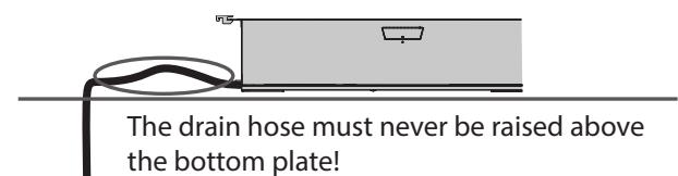
The drain hose must never be raised above the bottom plate!
