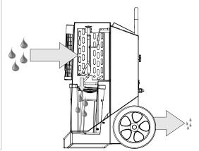
As the air is repeatedly circulated through the dehumidifier, its moisture content is repeatedly reduced, resulting in rapid, gentle drying. The dehumidifier can run constantly or be controlled by a built-in hygrostat.
