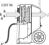
As the air is repeatedly circulated through the dehumidifier, its moisture content is repeatedly reduced, resulting in rapid, gentle drying. The dehumidifier can run constantly or be controlled by a built-in hygrostat.
